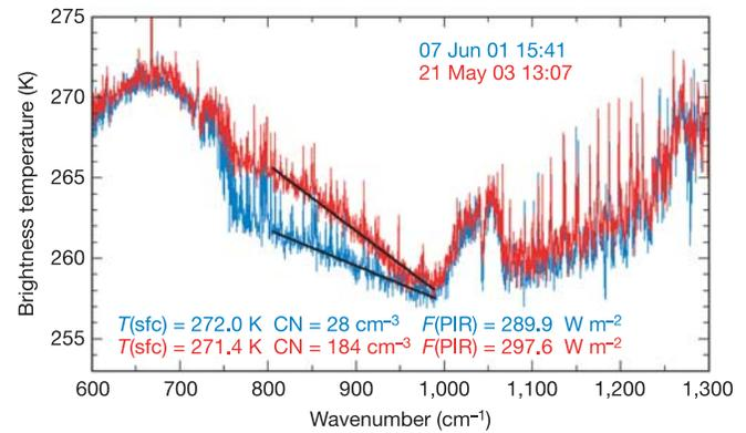
**Figure 2 | Examples of AERI measurements.** Downwelling emission spectra measured by the NSA AERI beneath two clouds with very different condensation nuclei (CN) concentrations. Near-surface air temperature  $T(\text{sfc})$  and pyrgeometer-measured downwelling longwave flux  $F(\text{PIR})$  are also indicated.
